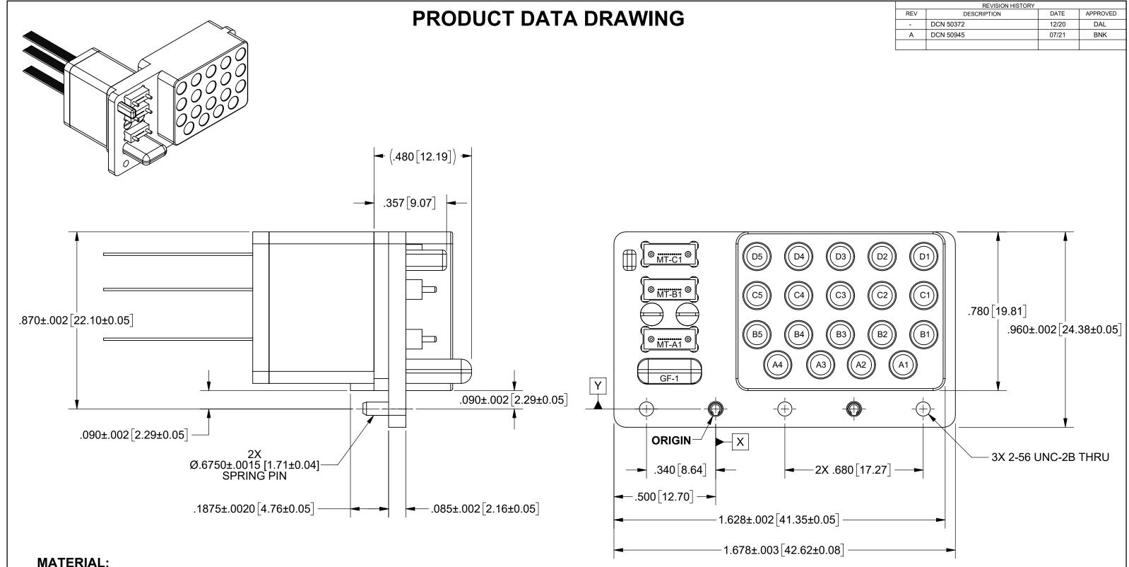
**BLOCK & RETAINERS:** STAINLESS STEEL PER AMS-5640, ALLOY UNS S30300, TYPE 1; OR ASTM A582 TYPE 303, COND. A
