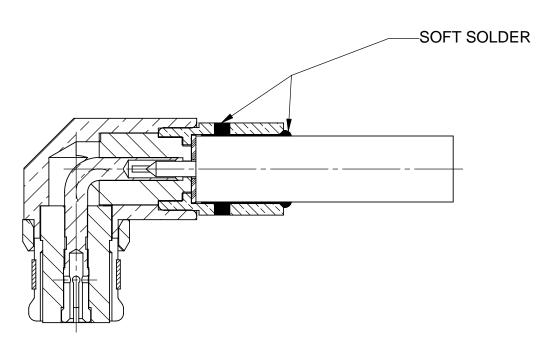
STEP 3: INSTALL CABLE INTO BODY AND SOFT SOLDER CABLE IN PLACE AS SHOWN.
